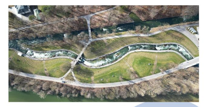
Length:308 m longDrop:4.1 mFlow rate:3 to 6 m/sec.Width:10 to 12 mDepth:40 to 120 cmGrade:WW IV - Safe rolling is required!
